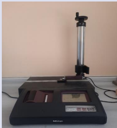
Figure 2: Profilometer device and surface roughness measurement.
