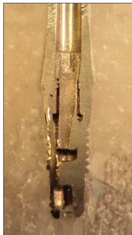
Figure 2. Cross-sectional view of IPH specimen.
