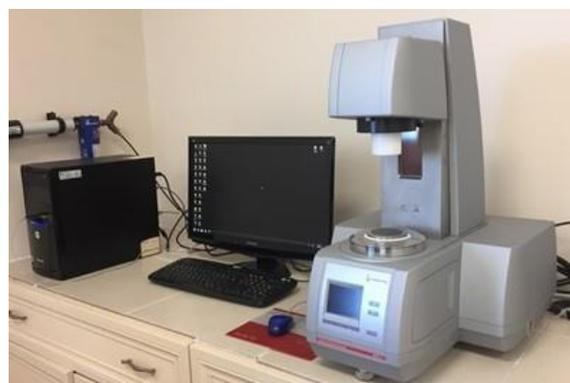
Figure 2. Anton Paar MCR 102 Rheometer.
