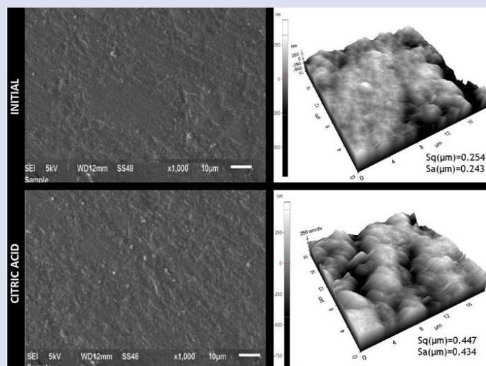
Figure 6: SEM and AFM images of BF composite resin initial and after immersion in citric acid.
