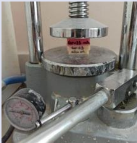
Figure 9. Pressing of the Ball Attachment System after Fastening
