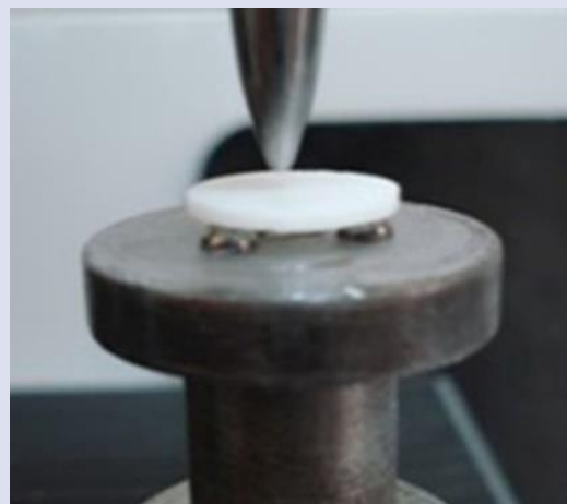
Figure 2. The sample was placed on stainless steel balls.
