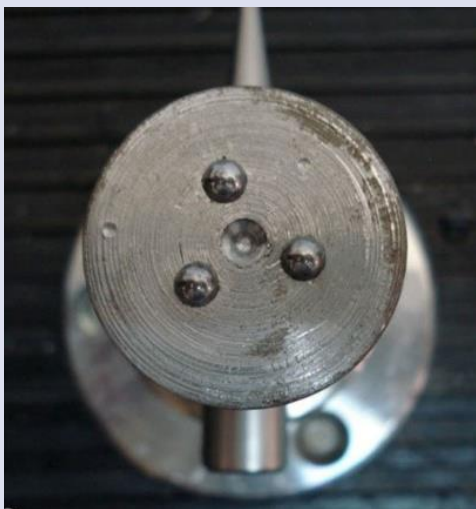
Figure 1. Positioning of stainless steel balls
