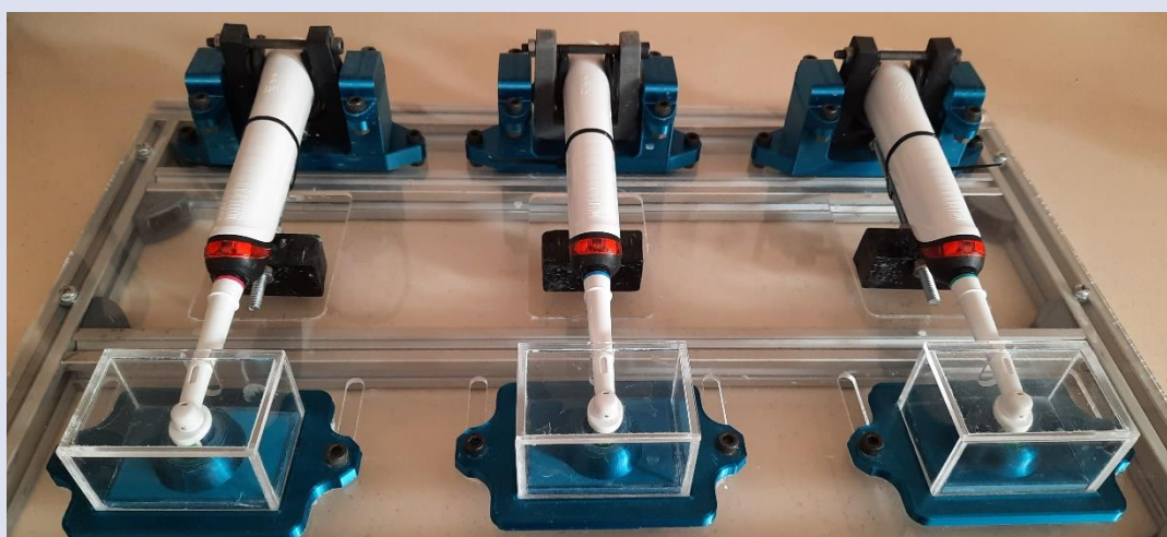
Figure 1: Brushing simulator used for brushing the samples.
