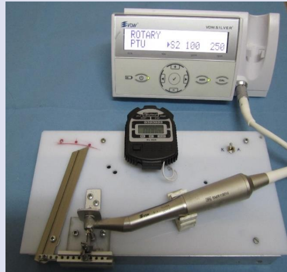
Figure 2. Test apparatus used for the evaluation of flexural fatigue
