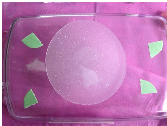
Figure1-a. The GC tissue conditioner located between two glass slabs with green acrylic stops,
