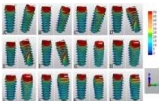
Figure 8. Von Mises stress distributions in anterior and posterior implants during oblique loading. Cr- Co / mesial 17° (A), Zirconia / mesial 17° (B), PEEK / mesial 17° (C), Cr- Co / distal 17° (D), Zirconia / distal 17° (E), PEEK / distal 17° (F), Cr- Co / buccal 17° (G), Zirconia / buccal 17° (H), PEEK / buccal 17° (I), Cr- Co / palatal 17° (J), Zirconia / palatal 17° (K), PEEK / palatal 17° (L).
