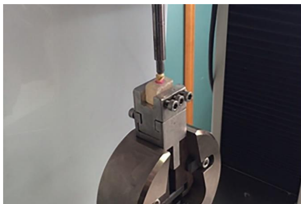
Figure 2. Fitting the acrylic block on the test device
