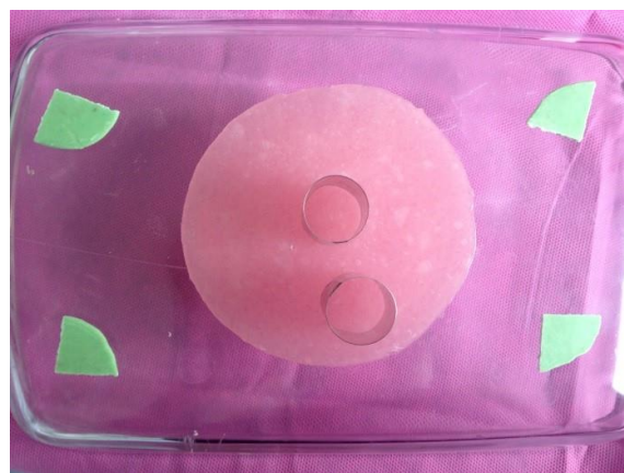
Figure1-c. Discs prepared by a group of tissue conditioners inside artificial saliva solution.
