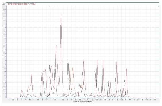
Figure 4. Comparison of HPLC solvents: Chromatograms of the HPLC solvent of 100 ng/g spiked sample with and without Oxalic acid
