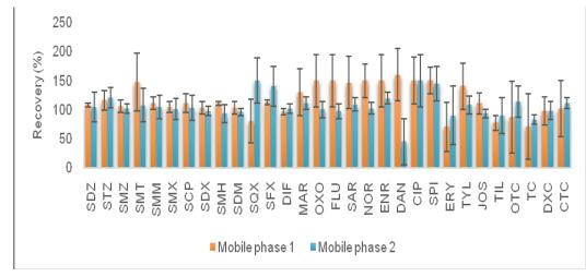
**Figure 3**. Effect of changes of extraction solvents on analytes. Mobile phase 1 -A 0.02% Formic acid and 1 mM Oxalic acid in deionized water, B- Acetonitrile 0.01% Formic acid, Mobile phase 2 -A 0.02% Formic acid in deionized water Mobile phase B Acetonitrile 0.01% Formic acid comparison.
