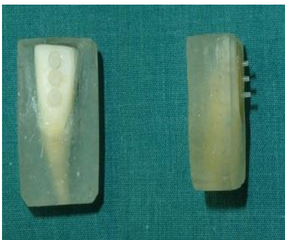
Figure 1. Three or two cylinders were obtained for the microshear bond strength test in each Specimen
