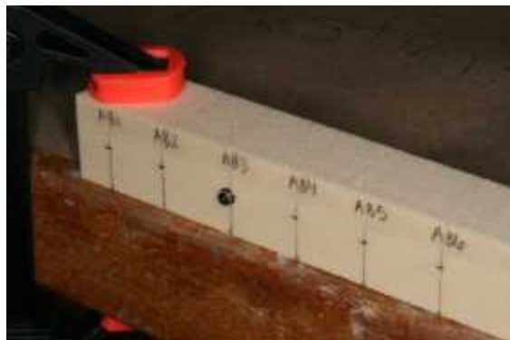
Figure 1. The mini-screws were randomly inserted at a 90-degree angle into custom-made synthetic bone blocks.
