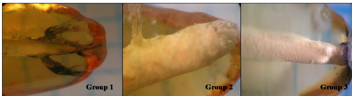
Fig. 1. Representative stereoscopic photographs from group 1 (2.5% NaOCl-CLC), group 2 (17% EDTA-CLC) and group 3 (Nd:YAG-CLC), original magnification 6X.
