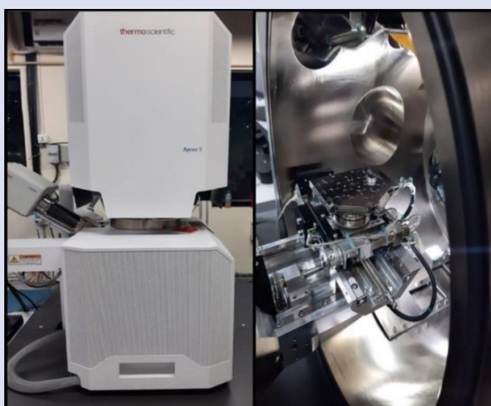
Figure 1. Quantitative analysis of surface topography using the FESEM with EDS
