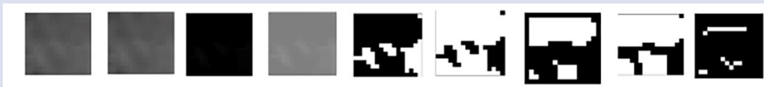
Figure 3: Fractal analysis steps: a- Saving and copying ROI images in 8-bit format after cropping, b- Images were duplicated and Gaussian filter (Sigma 35 pixels) applied. c- Applying 'subtraction' process to the image. d-128 gray values were added to each pixel and the threshold value was determined as 128. e- Converting the resulting image into binary format. f- Erosion application to images g- Dilation application h- Image reversal i- Skeletonization of the resulting image
