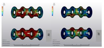
Figure 1. Von Mises stresses in plates a) Titanium b) CFR-PEEK
