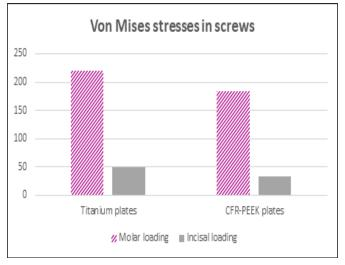
Figure 3. Von Mises stresses in screws
