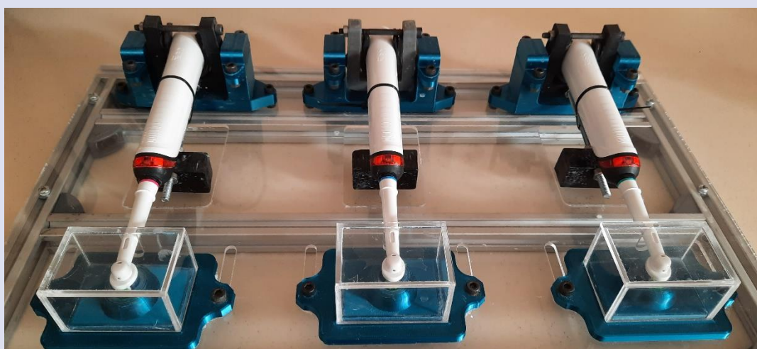
Figure 1: Brushing simulator used for brushing the samples.
