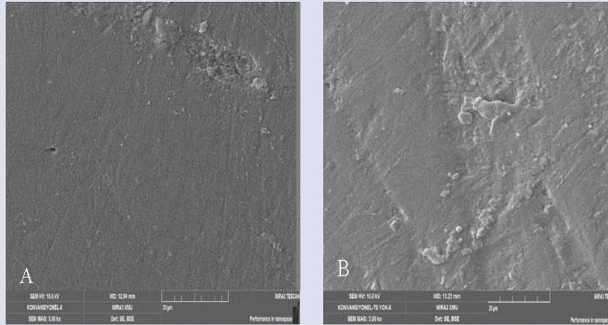
Figure 3: Image of surface properties of samples obtained by Conventional at x5000 magnification under SEM. A: No-thermocycling, B: Thermocycling.
