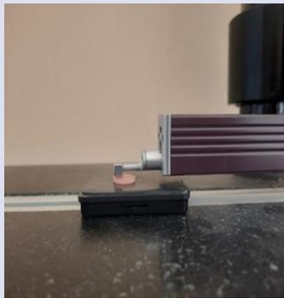
Figure 2: Profilometer device and surface roughness measurement.
