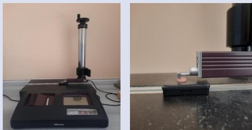
*Figure 2: Profilometer device and surface roughness measurement.*
