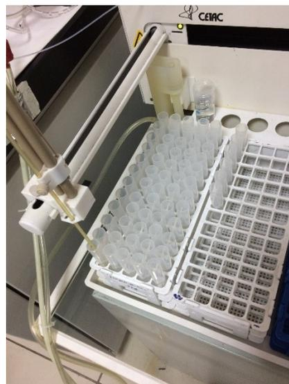
Figure 3. ICP-MS device when reading samples
