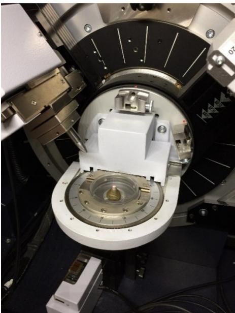
Figure 4. A disc in the XRD device holder
