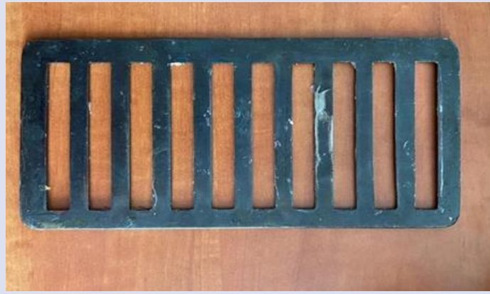
Figure 1. Stainless steel mold used to repair specimens.
