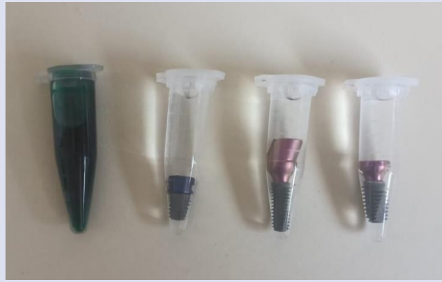
Figure 3. Solution of dyestuff in water (left) and symbolic representation of sealing experiments.
