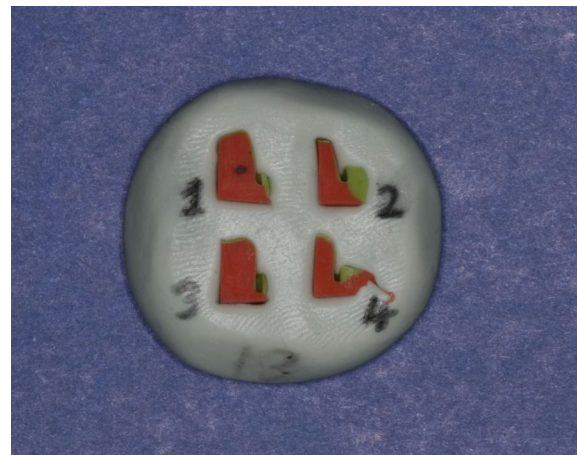
Figure 3: Sectioned replicas were embedded in putty impression material to stabilize the measurement.
