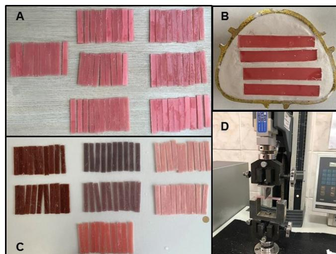
**Figure 1.** Experimental design of the study (A: 70 waxes, B: Waxes placed in muffles, C: Control and modified heat-cure acrylic resins, D: Flexural strength test).
