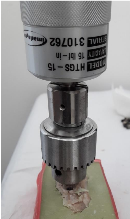
Figure 4: Illustration of RTV measurements which performed by digital torque meter.
